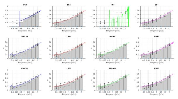
Fig. 7. Absorption coefficient of the melamine foam sample with a filtering process to minimize background noise. The labeling and distribution of the individual plots is the same as in Fig. 7.
