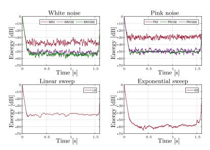
Fig. 11. ETC measured for the impedance tube using different excitation signals. White noise and pink noise were computed with 1, 100 and 1000 averages.
