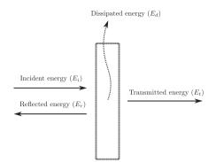
Fig. 1. Energy balance of the incident sound in a barrier. Adapted from [3,4].
