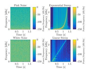
Fig. 4. Spectrogram of recorded stimulus signals during the measurement of the absorption coefficient in the impedance tube.
