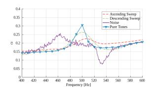
Fig. 8. Discontinuity on the  $\alpha$  measurement system for 400 Hz to 600 Hz frequency band.
