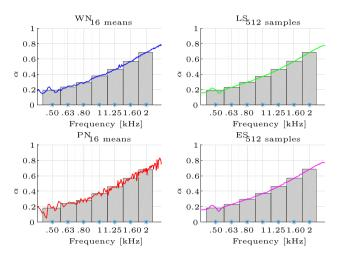
**Fig. 10.** Absorption coefficient  $\alpha$  results for the second experiment. All curves present the same frequency resolution and were obtained with excitation signals of same duration.
