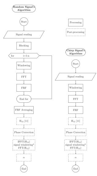
**Fig. 5.** Signal processing and post-processing algorithm for random and sine sweep inputs. \*The windowed signal size is not reduced using the first set while it is reduced to 512 samples in the second set.
