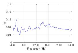
**Fig. 9.** Empty tube  $\alpha$  measurement, from [26].
