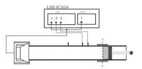
**Fig. 3.** Experiment configuration using an impedance tube with the two microphone technique and a LMS SCADA as the signal generator (OUT, channel 1) and processing equipment (IN, channels 1–3).
