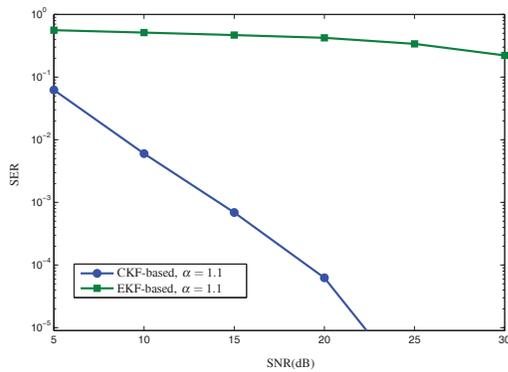
Fig. 4: Symbol error rate for detected symbols using aging factor.
