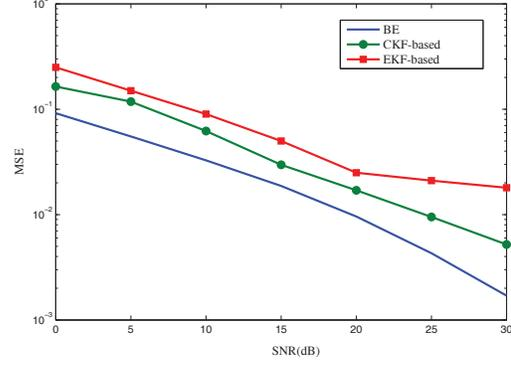
Fig. 1: Mean square error of channel tracking for  $f_D T = 0.01$ .
