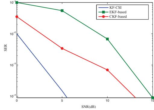
Fig. 2: Symbol error rate for detected symbols for  $f_D T = 0.01$ .
