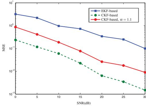
Fig. 3: Mean square error of channel tracking for  $f_D T = 0.005$ .
