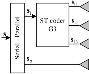
Fig. 2. Architecture of the HMTS G3+1 transmitter
